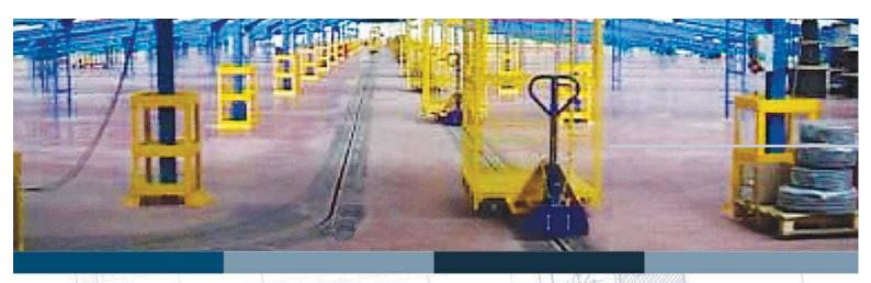
The **transport vehicles** most commonly used in the TOW-LINE system are pallet loaders and trolleys equipped with a tow mechanism, a safety system in case of collision, and a code rack (in the case of manual scanning) or a TAG support (for automatic – RFID reading).
